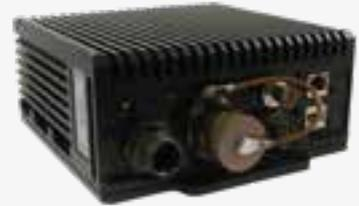
This Tri-Band version of the 5RM unit, offers support for high L-band, S-band and C-band.
