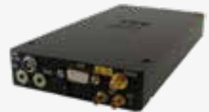
The SOL8SDR2x2W-P is a 2x2 watt MiMo Mesh radio in a practical enclosure suitable for desktop use or platform integration and incorporating industry standard interface connections.
