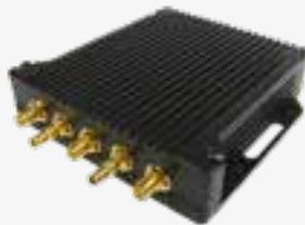
The SOL8SDR-R offers the same feature set and 2x100mW output power as the SOL8SDR-C but in a rugged form factor with military standard connectors. Ideal for bench testing, platform integration or as a low power soldier data radio.
